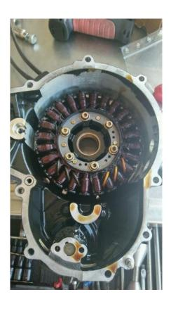
All Rotax engines produce electricity from a Stator. The stator works off the engine crank shaft and is the most dependable source of electricity in general aviation. The stator produces 18 amps.
