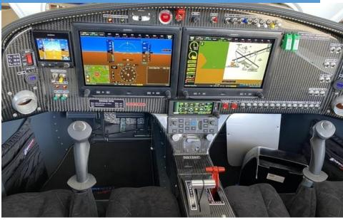
All Bristells LSA's can be registered as an ELSA and flown IFR in IMC if the pilot has a medical and is IFR rated. The plane is required to have an IFR certified piece of avionics, such as the GNX 375 GPS with LPV vertical guidance.
