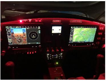
This Bristell 912iS Sport is equipped with dual G3X 10-inch Touch Screens, a Back up G5, and a Val 2000 Certified ILS receiver. If the owner changes it to an ELSA, it can be flown IFR in IMC.
