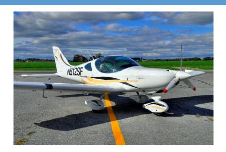
Ground Adjustable Prop can be set to match the owner's preference. Coarse for high cruise speed and fine for great climb rate.
