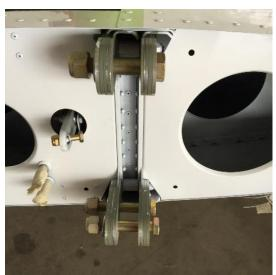
Massive wing bolts attach to the spars. Bristells are very strong with a Vne of 157 KIAS.
