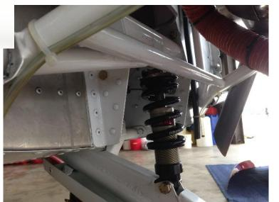
The nose wheel has dual shock absorbers. A center hydraulic cylinder and an outer steel coil spring.
