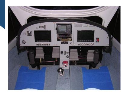
Rudder pedal handle adjusts pedals forward for short pilots and back for tall pilots
