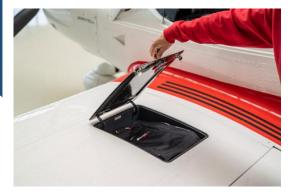
The wing spar extends 14 inches beyond the fuselage, so pilot does not step on the wing or over a flap. The wing attaches where the red paint ends.
