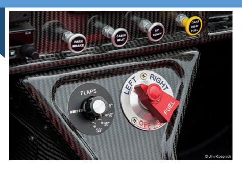
The knob on the left is the parking brake. The Cabin heat works great due to the tight-fitting canopy. The UP/DOWN knob directs heat to your feet or to the canopy for defrost. The carburetor heat knob is yellow.
