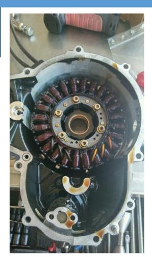
All Rotax engines produce electricity from a Stator. The stator works off the engine crank shaft and is the most dependable source of electricity in general aviation. The stator produces 18 amps. The Bristell 915 Turbo has dual stators.
