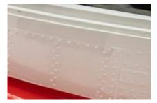
The 3400 rivet heads are filled with epoxy, sanded and painted to prevent corrosion and result in a professional looking aircraft.
