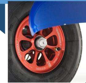
The Berringer Wheels and Brakes enhance Safety because they are anti-lock and anti skid. The bearings are sealed and last 7 years. The wheels do not need to be removed during the annual inspection reducing cost and wear.
