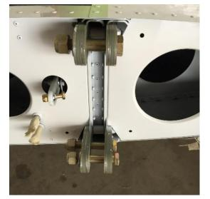
Massive wing bolts attach to the spar both forward and aft. All Bristells have a Vne of 157 KIAS. This is one strong airplane.
