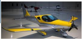
Bristells are constructed of tried-and-true aluminum. The aluminum is 6061 grade, the same as used on the space shuttle. Milan Bristela, the CEO and Aeronautical Engineer that designed Bristell, decided to use 4 grades of aluminum to keep the weight low. . Carbon fiber is also used to save weight.
