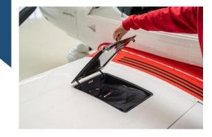
The wing spar extends 14 inches beyond the fuselage, so pilot does not step on the wing or over a flap. The wing attaches where the red paint ends.
