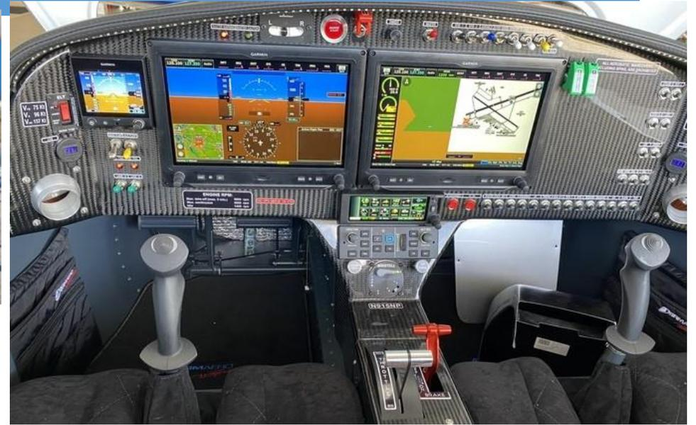
**All Bristells LSA's can be registered as an ELSA and flown IFR in IMC if the pilot has a medical and is IFR rated. The plane is required to have an IFR certified piece of avionics, such as the GNX 375 GPS with LPV vertical guidance.**
