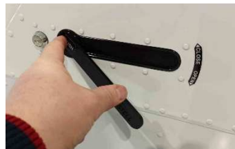
2. Push lever tip and turn lever down
