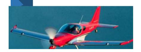
100 HP ROTAX with dual aneroid carburetors and dual electric starting packs. Stator for dependable 18 amp electrical output. When set at reduced throttle of about 5000 RPM will result in a 4 GPH fuel burn of , 93 octane premium Autogas
