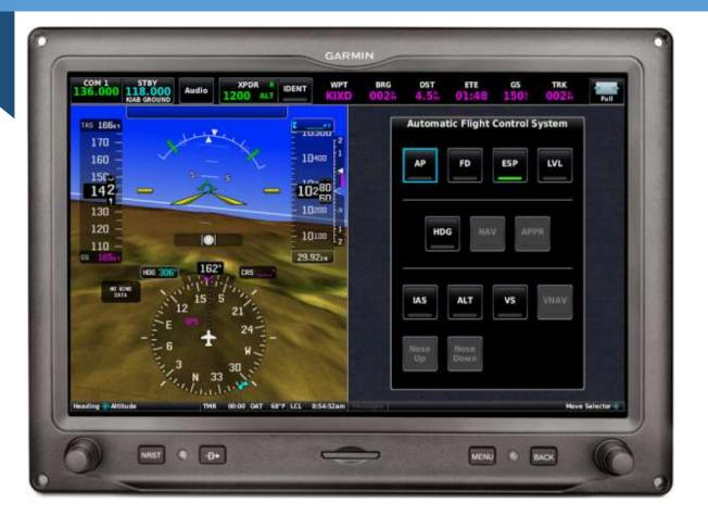
The Com is displayed in the upper left-hand corner. Touching the blue, STBY box will place the STBY frequency in the Com 1 Box.
