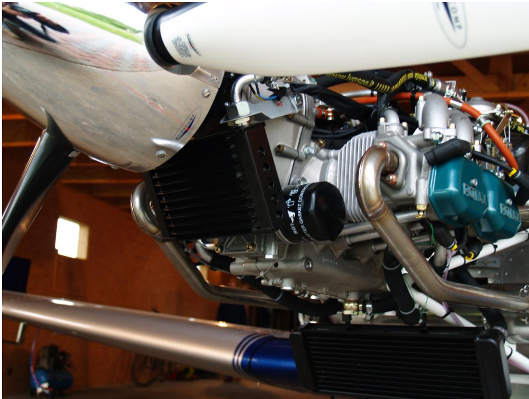
Fig. 10-14: Attachment of the radiator on the engine
